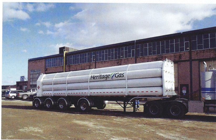
The low cost of natural gas is making it feasible for Heritage Gas to bring CNG to remote locations via tube trailer on a long-term basis.
